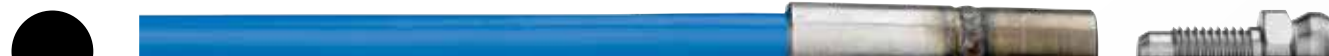
Midsize Thermoplastic (5/4) P/N: 51953 0.590" OD for 0.715" ID or larger tubes. Blue plastic covering (previously Gray) with 3/8"-24 RH female threaded, SS end fittings on both ends. Also available with 9/16" Type M inlet fitting. Use JETSTREAM type HPM nozzles. Smallest end fitting diameter in the industry with 26,100 psi working pressure with lengths up to 300'. Temperature rating of -22°F to 140°F (-30°C to +60°C).
