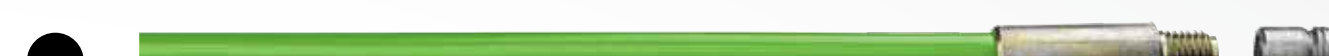
Small Thermoplastic (4/2) P/N: 26104 0.394" OD for 0.519" ID or larger tubes. Green plastic covering (previously Red) with 1/16" NPT male end fittings on both ends. Has a higher burst rating than Part No. 50559, but with less flexibility. Use JETSTREAM type FP, FCC, FPT, E & EX nozzles. 17,400 psi working pressure with lengths up to 300'. Temperature rating of -22°F to 140°F (-30°C to +60°C).
