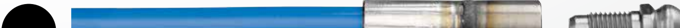
Large Thermoplastic (8/4) P/N: 53816 0.795" OD for 0.920" ID or larger tubes. Blue plastic covering (previously Gray) with 9/16"-18 RH female threaded, SS end fittings on both ends. Also available with 3/4" Type M inlet fitting. Use JETSTREAM type HPM nozzles. Smallest end fitting diameter in the industry with 21,750 psi working pressure with lengths up to 300'. Temperature rating of -22°F to 140°F (-30°C to +60°C).
