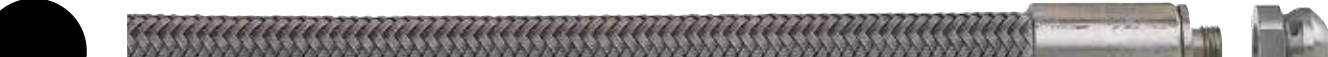
Compact Nozzle C-2 P/N: 50752 0.565" OD for tubes 0.690" ID or larger. High pressure antistatic smoothbore PTFE tube with maypole and spiral wound high tensile 304 SS with a special nozzle thread on one end and a 1/8" NPT inlet fitting on the opposite end. The special end fitting allows for use with Jetstream C-2 nozzle. 10,000 max operating pressure in lengths up to 50'. Temperature rating of 76°F to 500°F (-60°F to 260°C).
