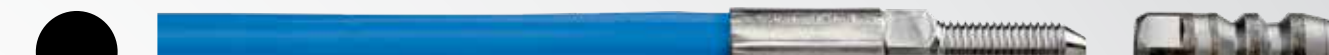
Midsize Thermoplastic (5/4) P/N: 51953 0.590" OD for 0.715" ID or larger tubes. Blue plastic covering (previously Gray) with 3/8"-24 LH or RH male threaded nozzle end and standard 9/16" Type M inlet fitting. Use JETSTREAM type HPF & HPE nozzles. 26,100 psi working pressure with lengths up to 300'. Temperature rating of -22°F to 140°F (-30°C to +60°C).
