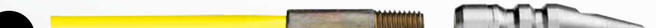
Large Thermoplastic (8/2) P/N: 27560 0.70" OD for 0.825" ID or larger tubes. Yellow polyurethane covering (previously Blue) with 3/8" NPT male end fittings on both ends. Use JETSTREAM type FP, FCC, FPT, E & EX nozzles. 12,180 psi working pressure with lengths up to 300'. Used primarily with Automation tools. Temperature rating of -22°F to 140°F (-30°C to +60°C).
