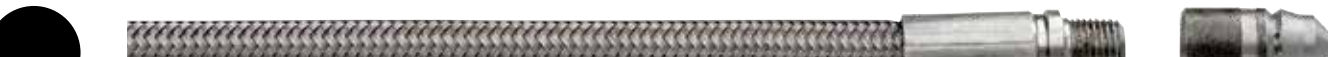
The Cleaning Contractor's Favorite! P/N: 25568 0.500" OD for tubes as small as 0.625" ID. Highly flexible and fast running SS braid reinforced with teflon core and 1/8" NPT male on both ends. Use Jetstream FP, FCC, FPT, E, & EX nozzles. 8,000 max operating pressure with lengths up to 50'.
