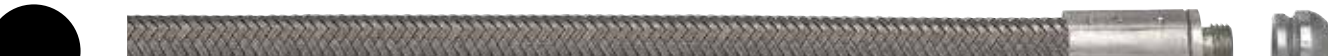
Compact Nozzle C-1 P/N: 50673 0.500" OD for tubes as small as 0.625" ID or larger. High pressure antistatic smoothbore PTFE tube with braided high tensile 304 SS with a special nozzle thread on one end and a 1/8" NPT inlet fitting on the other. The special end fitting allows for use with Jetstream C-1 nozzle. 8,000 max operating pressure in lengths up to 50'. Temperature rating of -76°F to 500°F (-60°C to 260°C).
