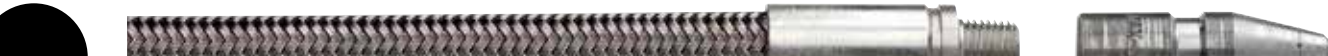
A Workhorse! P/N: 25570 0.575" OD for tubes as small as 0.700" ID. Best overall lance in its size range. Highly flexible teflon core with four layers of SS wire braid/spiral wraps and 1/8" NPT male on both ends. Use Jetstream FP, FCC, FPT, E, & EX nozzles. 10,000 max operating pressure with lengths up to 50'.
