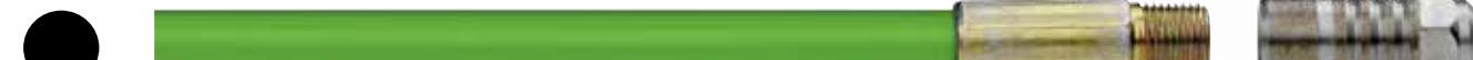
Midsize Thermoplastic (5/2) P/N: 26106 0.508" OD for 0.633" ID or larger tubes. Green plastic covering (previously Blue) with 1/8" NPT male end fittings on both ends. Has a higher burst rating than Part No. 25568, but with less flexibility. Use JETSTREAM type FP, FCC, FPT, E & EX nozzles. 15,080 psi working pressure with lengths up to 350'. Temperature rating of -22°F to 140°F (-30°C to +60°C).
