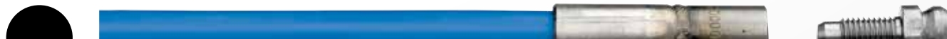
Midsize Thermoplastic (6/4) P/N: 51954 0.646" OD for 0.771" ID or larger tubes. Blue plastic covering (previously Gray) with 3/8"-24 RH female threaded, SS end fittings on both ends. Also available with 9/16" Type M inlet fitting. Use JETSTREAM type HPM nozzles. Smallest end fitting diameter in the industry with 21,750 psi working pressure with lengths up to 300'. Temperature rating of -22°F to 140°F (-30°C to +60°C).
