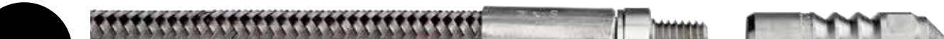
Big Bore Teflon Core P/N: 25571 0.721" OD for tubes 0.825" ID or larger tubes. Yellow polyurethane covering (previously Blue) with 3/8" NPT male end fittings on both ends. It has four layers of SS wire braid/spiral wraps and 1/4" NPT male on both ends. Use Jetstream FP, FCC, FPT, E, & EX nozzles. 10,000 max operating pressure with lengths up to 50'.
