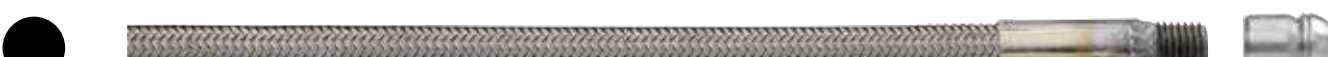
The Professional's Lance for Small Tubes P/N: 50559 0.340" OD for tubes as small as 0.465" ID. Highly flexible and fast running SS braid with teflon core and 1/16" NPT male on both ends. Use Jetstream FP, FCC, FPT, E, & EX nozzles. 8,000 max operating pressure with lengths up to 50'.
