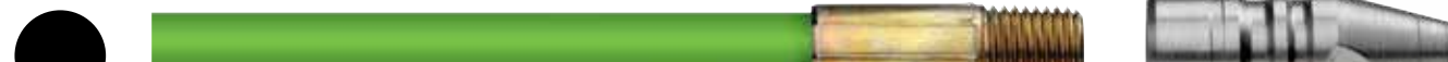
Midsize Thermoplastic (6/2) P/N: 26108 0.547" OD* for 0.672" ID or larger tubes. Green plastic covering with 1/4" NPT male end fittings on both ends. Has a higher burst rating than Part No. 25571, but with less flexibility. Use JETSTREAM type FP, FCC, FPT, E & EX nozzles. 15,950 psi working pressure with lengths up to 300'. Temperature rating of -22°F to 140°F (-30°C to +60°C).
