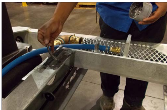
Figure 128: Apply Anti-Seize to the Pump Channels.
