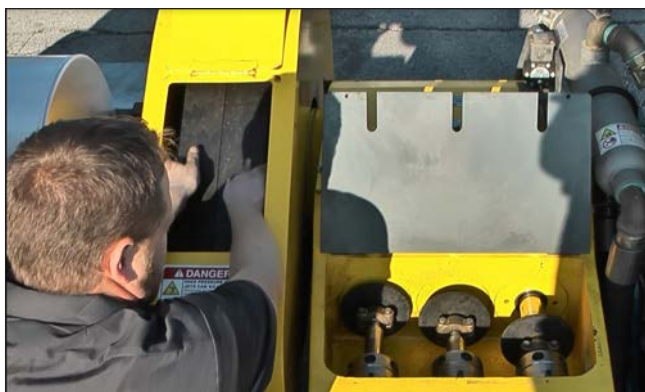
Figure 99: Rotating the Belt Drive.
