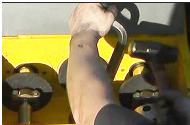
Figure 61: Tightening the Gland.
