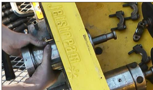
Figure 29: Stuffing Box Removal.
