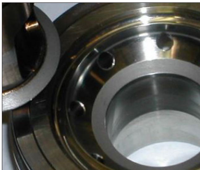
Figure 92: Properly Lapped Valve Seats.
