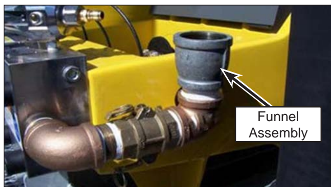
Figure 14: Funnel Assembly Installation.
