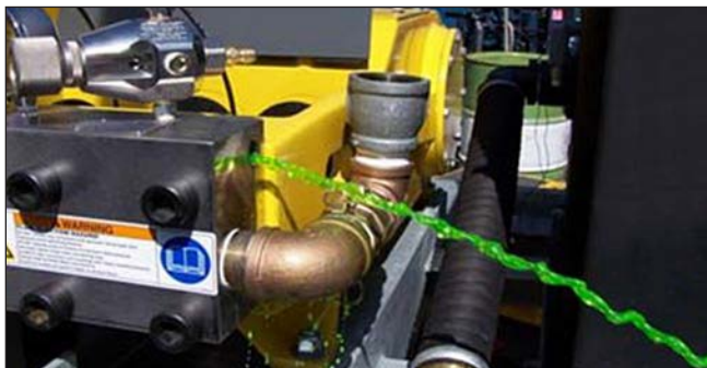
Figure 16: Draining the Anti-Freeze.
