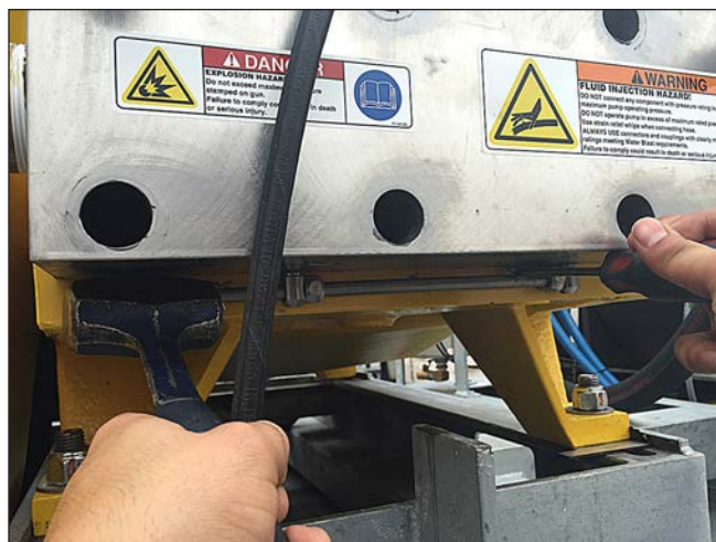
Figure 35: Hinge Rod Installation.
