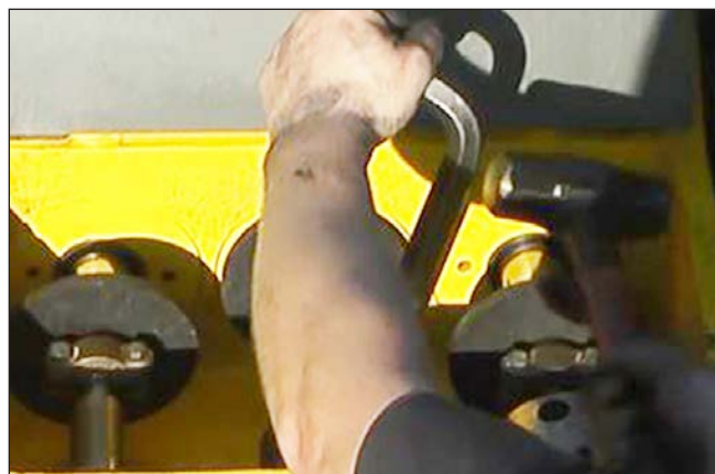
Figure 45: Tightening the Gland Nut.
