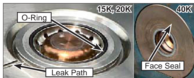
Figure 12: Uni-valve to Stuffing Box Seals.
