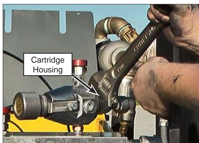
Figure 94: Cartridge Housing Removal.
