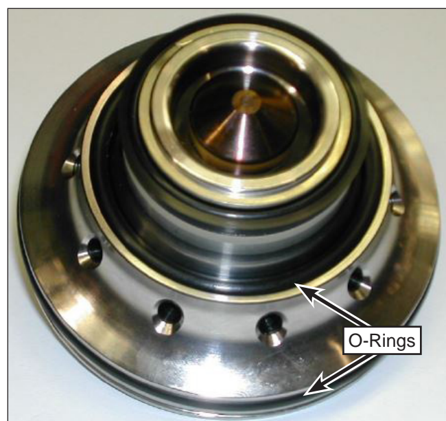
Figure 89: Install the O-Rings.
