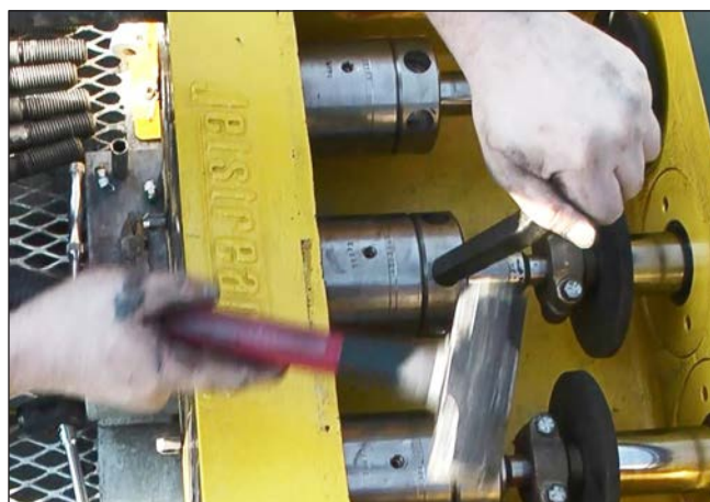
Figure 31: Tightening the Gland Nuts.
