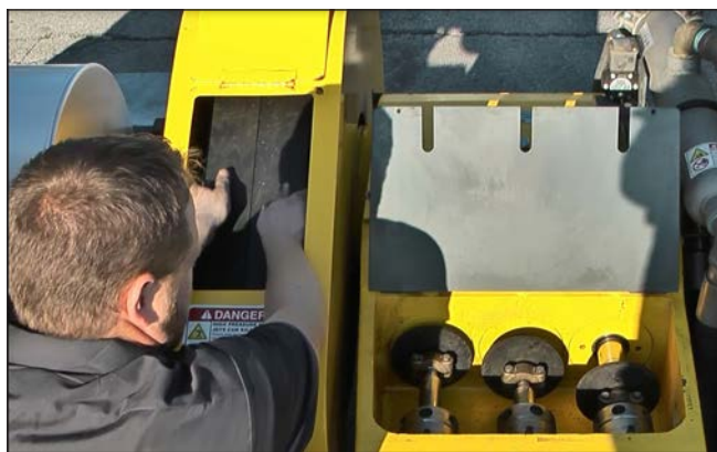
Figure 48: Rotating the Belt Drive.
