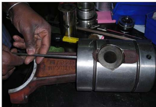
Figure 121: Set Screw Removal.
