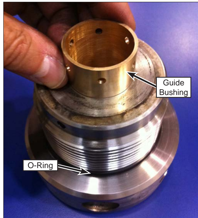
Figure 57: Guide Bushing Installation.
