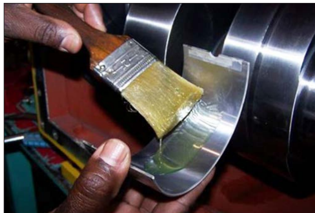
Figure 115: Lubricating the Bearing.
