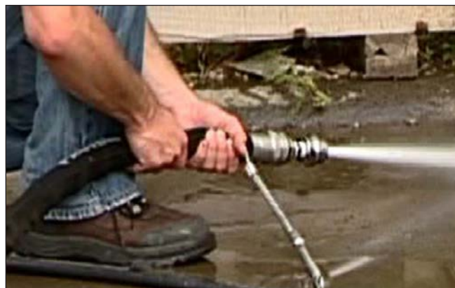
Figure 8: Flushing the Discharge Hose.
