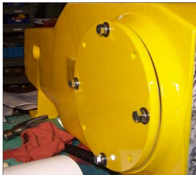
Figure 139: Side Plate Installation.
