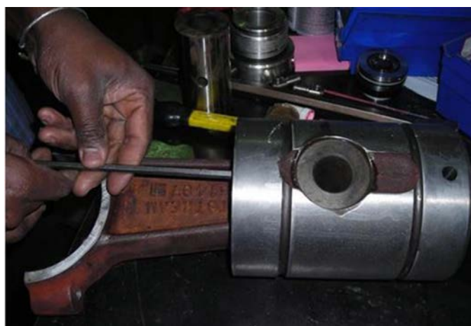
Figure 124: Second Set Screw Installation.
