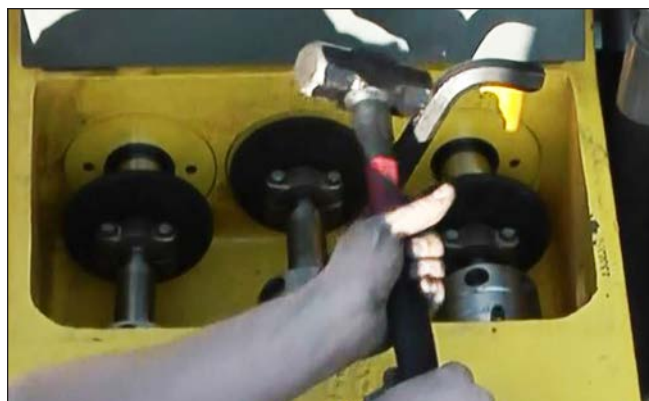
Figure 49: Loosening the Gland Nut.
