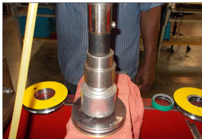
Figure 104: Pressing the Seal.
