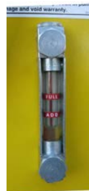
Fig. 115: Typical Oil Level for Recently Operated Pump
