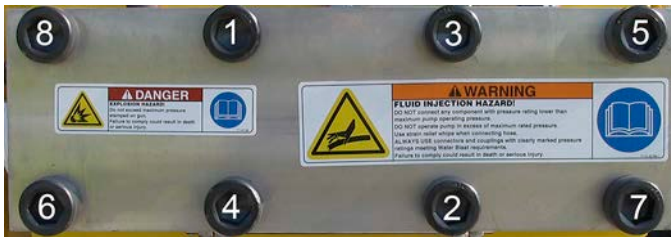
Fig. 86: Tightening Sequence
