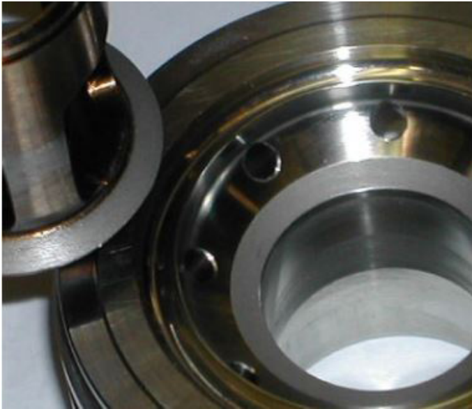
Fig. 109: Properly Lapped Valve Seats
