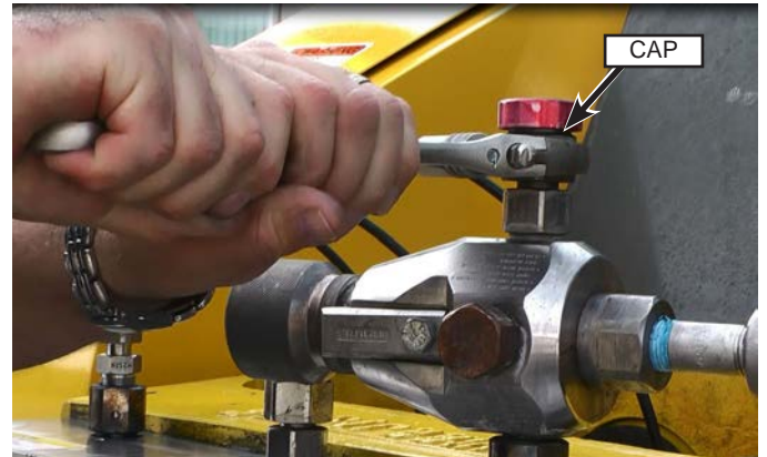
Fig. 63: Housing Removal (15K Manifold Shown)
