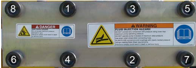
Fig. 61: Tightening Sequence
