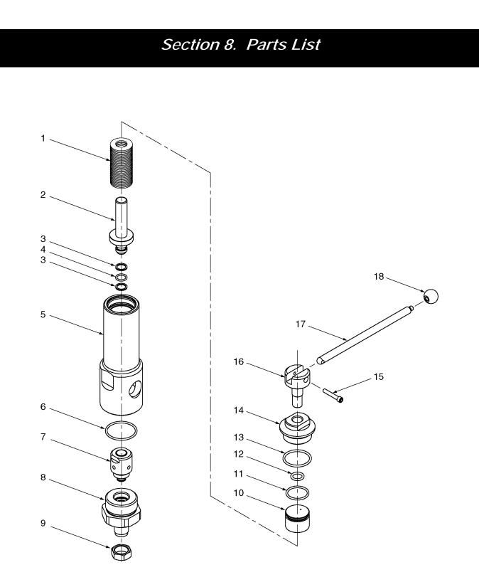
Figure 1-1. Hand-Adjustable Pressure Regulator Parts Diagram
