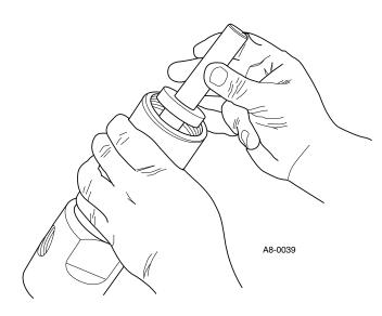
Figure 7. Spring Plunger Installation
