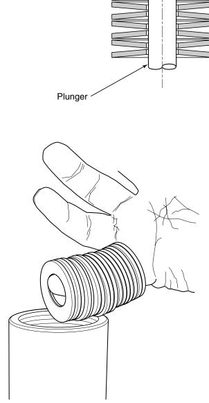
Figure 11. Stacking Disc Springs
