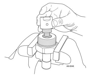
Figure 14. Installing Cartridge
