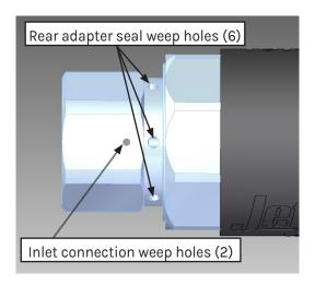
If a leak persists even after a cartridge replacement, the main shaft female cone may be damaged and require replacement. (A new cartridge may drip and will require a high pressure cycle - on/off a few times - to get the cartridge shaft to seat to the main shaft. If this does not stop the leak, use a small tool to push on the rear of the cartridge shaft to press the small shaft into the main shaft.) See Section 7.0, Troubleshooting, for more information.
