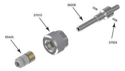
An interim solution is available to replace only the seal kit (PN 65445) portion of the seal cartridge. If replacing only the seal kit still results in leakage, full seal cartridge may need to be replaced.
