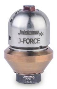
The 2" J-Force™ is a self-powered rotating nozzle designed to easily navigate and clean 2" pipes with up to 90° bends. The 2" J-Force has front, side, and rear jets that clear blockages, clean, and provide thrust to propel the tool down the pipe for maximum cleaning power and minimum wear.
