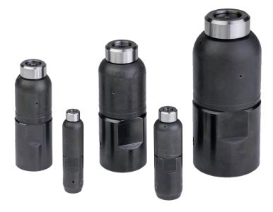
The DrillJet<sup>™</sup> is a self-powered rotating nozzle designed for tube cleaning available in five sizes with a variety of inlet options. The DrillJet<sup>™</sup> is a universal type of tool with six or seven nozzles that clear blockages, clean, and provide thrust to propel the tool down the pipe. The tool is available in a range of pressures and flows depending on size.
