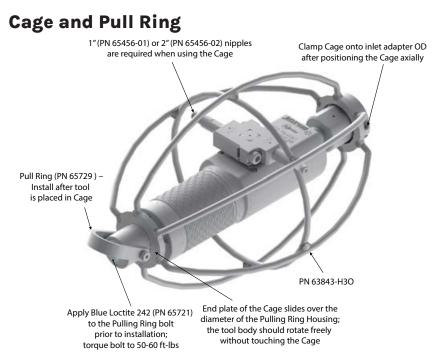
**NOTE:** Only 1" or 2" extensions can be used when the  $H_3$ Orbiter is installed in the centralizer. Pull ring and Inlet adapter required to secure the  $H_3$ Orbiter in the cage.
