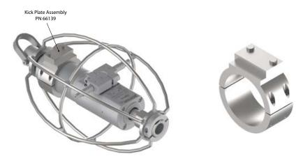
**NOTE:** Effectiveness of the kick plate is dependent on tool setup (nozzle/manifold) and material in pipe. At 20K operation, a minimum flow of 17 gpm with the R90 manifold is recommended. Use of the R150 manifold with the kick plate assembly is not recommended.
