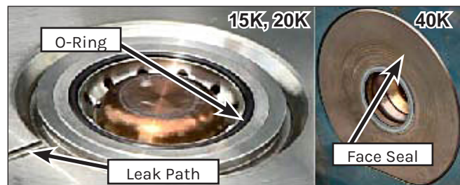
Figure 41: Uni-valve to Stuffing Box Seals.
