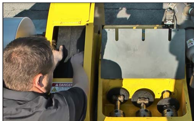
Figure 85: Rotating the Belt Drive.
