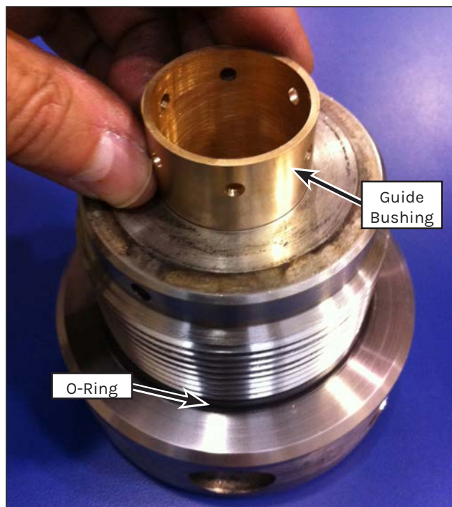
Figure 89: Guide Bushing Removal (15K/20K Gland Nuts).
