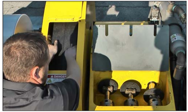
Figure 145: Rotating the Belt Drive.
