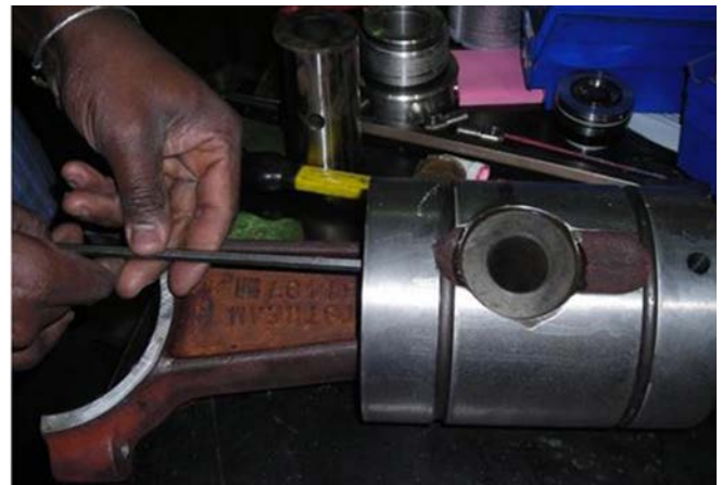
Figure 171: Second Set Screw Installation.
