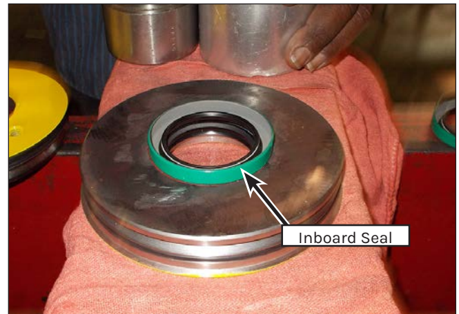
Figure 152: Inboard Seal Installation.
