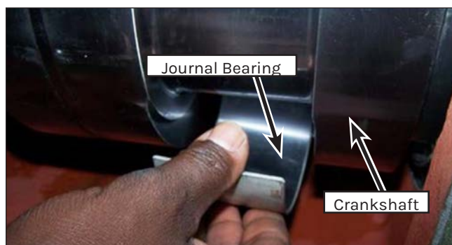
Figure 163: Rod Bearing installation.
