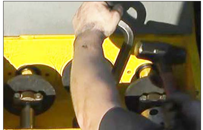
Figure 83: Tightening the Gland Nut.
