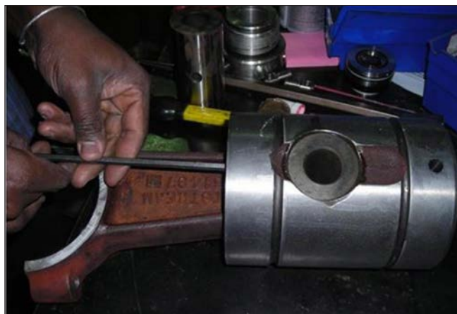
Figure 168: Set Screw Removal.
