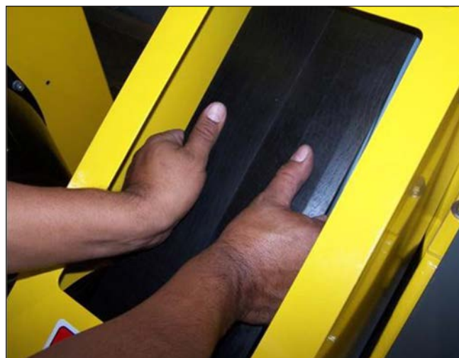
Figure 157: Rotating the Pump.
