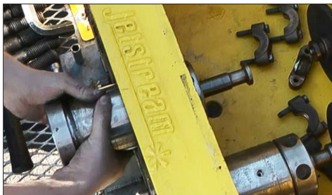
Figure 67: Stuffing Box Removal.
