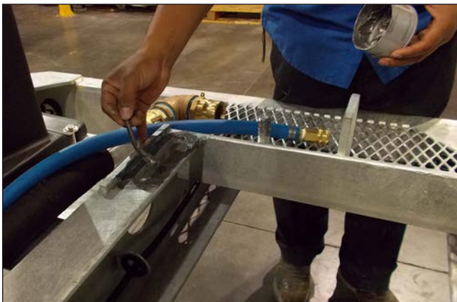
Figure 175: Apply Anti-Seize to the Pump Channels.
