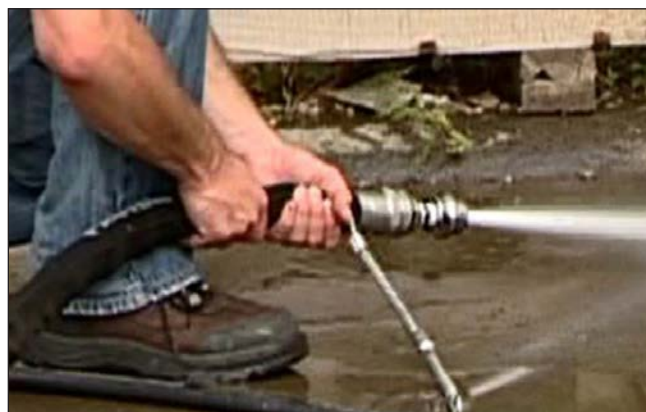
Figure 34: Flushing the Discharge Hose.
