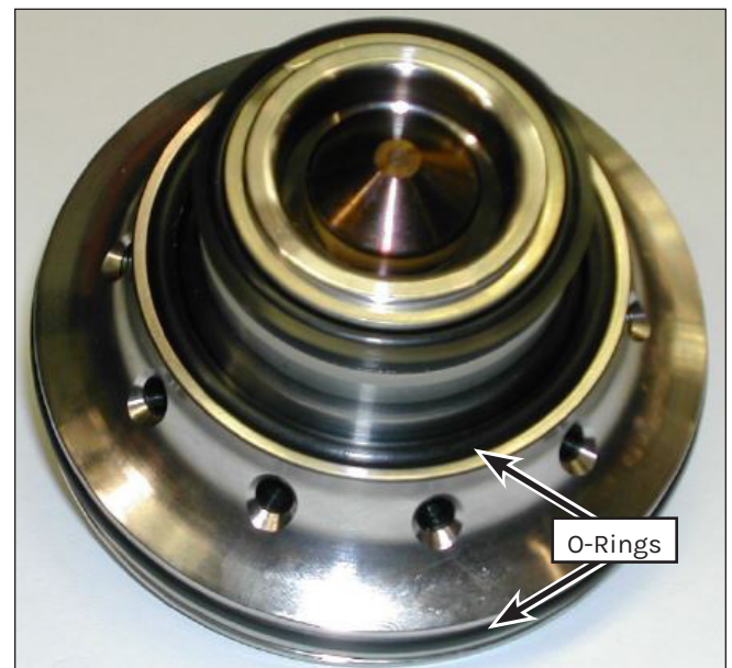
Figure 127: Install the O-Rings.
