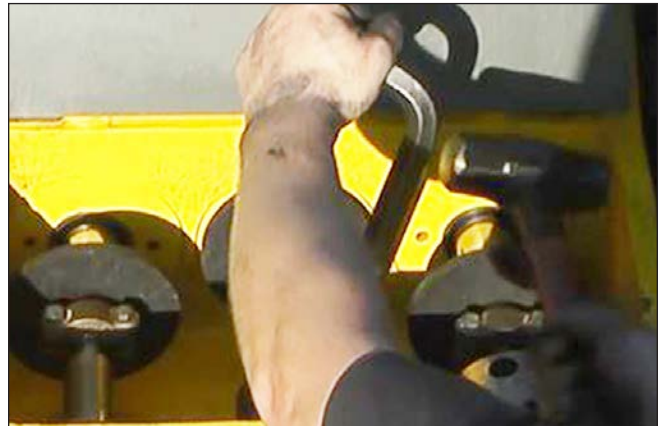
Figure 99: Tightening the Gland.
