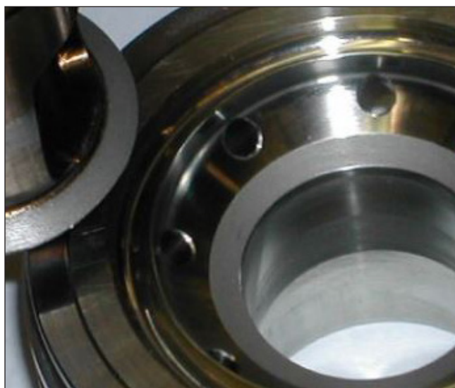
Figure 130: Properly Lapped Valve Seats.
