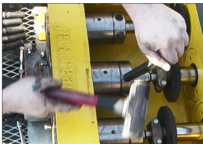
Figure 69: Tightening the Gland Nuts.
