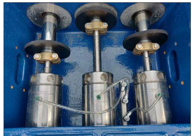
Figure 37: 5200 Series Water Lubrication System.
