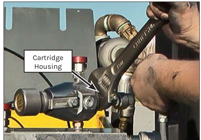
Figure 132: Cartridge Housing Removal.
