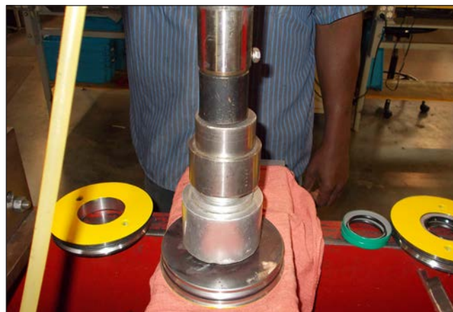
Figure 151: Pressing the Seal.
