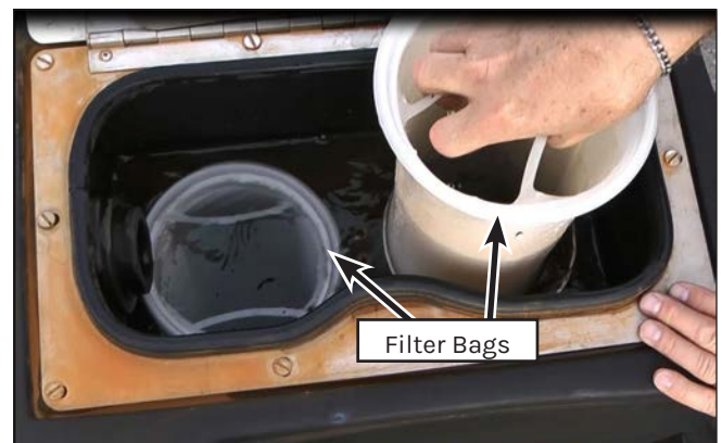
Figure 54: Filter Bag Removal.
