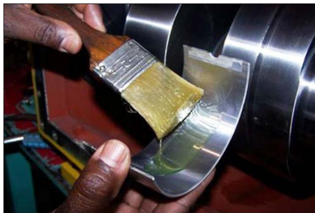
Figure 162: Lubricating the Bearing.
