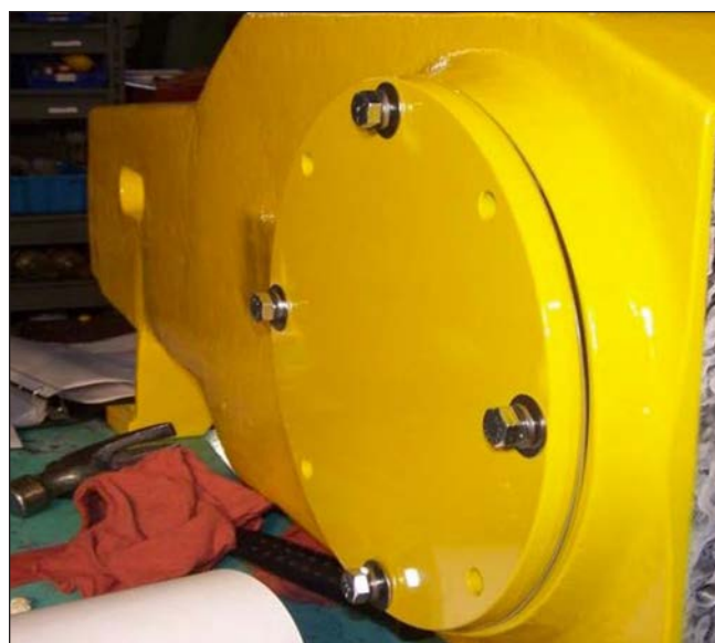
Figure 186: Side Plate Installation.
