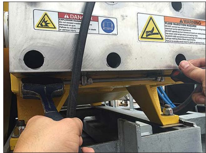
Figure 73: Hinge Rod Installation.
