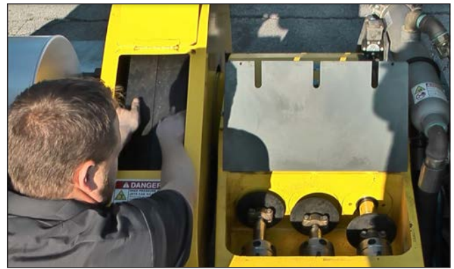
Figure 146: Rotating the Belt Drive.
