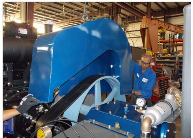
Figure 142: Belt Guard Removal.
