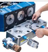
UNMATCHED VERSATILITY: The UNx<sup>™</sup> Fluid End system simplifies maintenance and allows for fast on-site conversions from 6,800 to 40,000 psi operating pressures, without the need for special tools, equipment, or torque.
