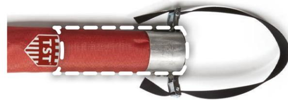
Closest to the lance, where the hose is most likely to break, there is a 250 mm / 9.8 in. solid steel collar, which effectively protects the operator in the event of an accident.
